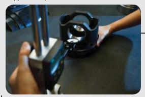
Cylinder liner dimensional control includes dozens of critical specifications, including inside and outside dimensions, flange specifications and origing groove size checks, which is accomplished through tools such as a CMM, height gauge, hardness testor and surface analyzer.
