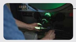
Shown here is our in-house tangential piston ring tension tester.
